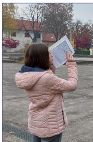
Figure 29 Measuring tree height using a clinometer
